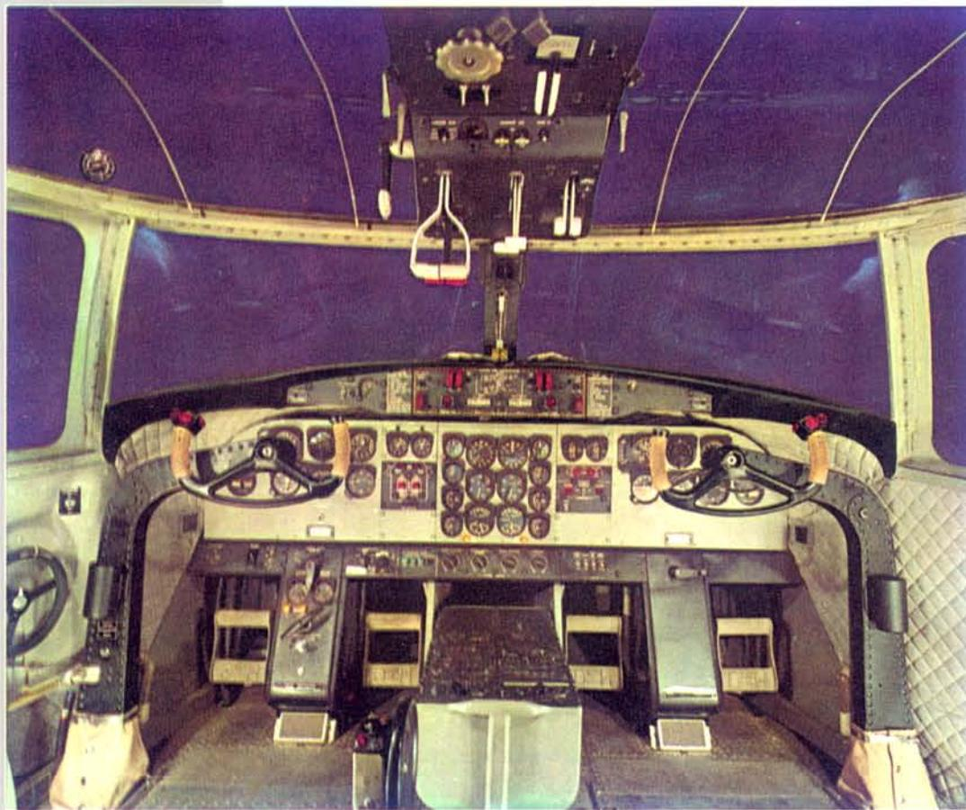
The nerve centre of the Caribou — the cockpit — is comprehensively equipped, but remains simple and functional. A main consideration is crew comfort and freedom of movement. All operational controls are within easy reach.
